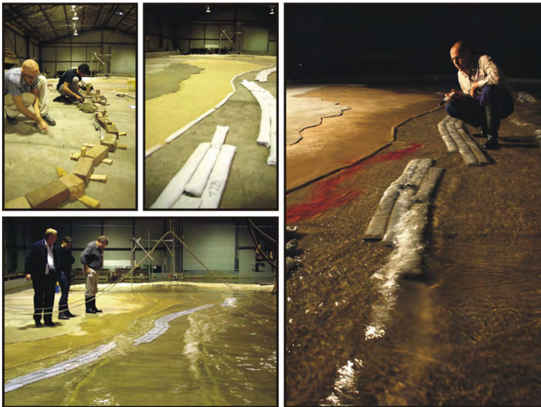
(Clockwise) Model construction – wave basin; Completed model before testing; Dye tracer testing - wave basin; Overtopping testing - wave basin
